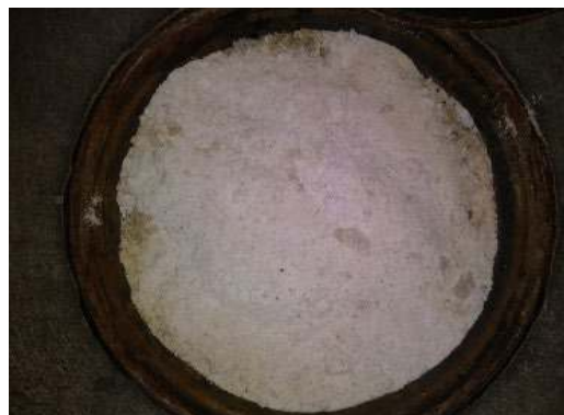
Appearance after absorbing H 2 S odors (100ppm+) for 30 days
