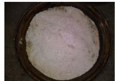
Manhole insert after absorbing H 2 S odors (100ppm+) for 30 days
