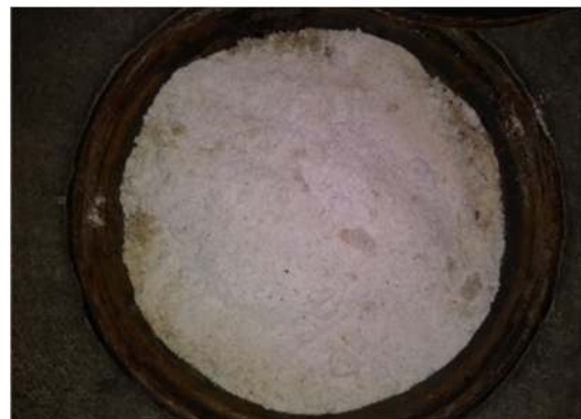
Appearance after absorbing H 2 S odors (100ppm+) for 1 Month
