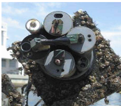
Biofouling build-up on marine data collection instruments with Fortify Sealer™ after 150 days.
