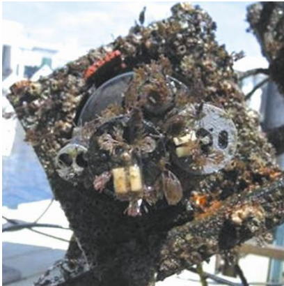
Biofouling build-up on marine data collection instruments without Fortify Sealer™ after 30 days.
