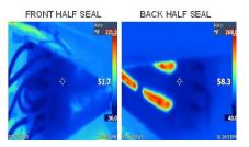
Large thermoplastic mold IR image **before** cooling channels cleaned with **Dr. KlarX™ Calci-Cure**.
